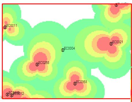
Compensation done using cell 255 and 321 Azimuth of the two cells also adjusted for optimal compensation
